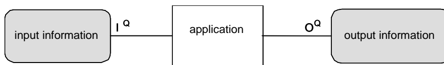
Fig. 4: Application including input information and output information as basic elements of information flowchart
